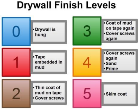
Figure 47: Drywall Finish Levels
